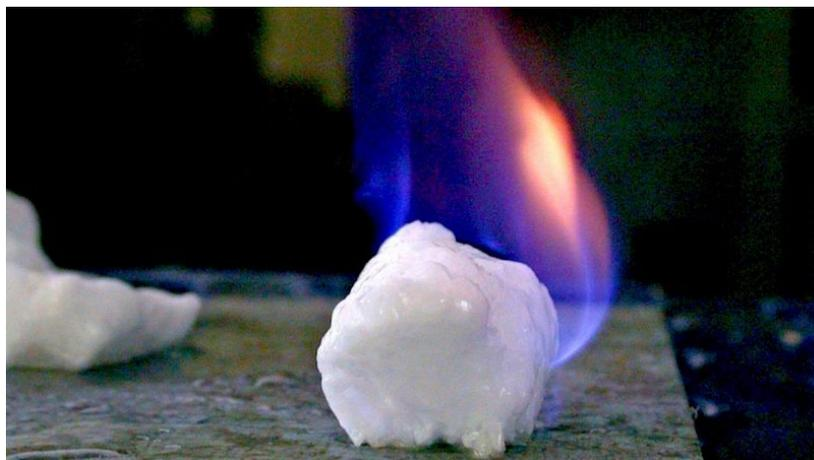
**Fig.2.** Example of flammable ice
